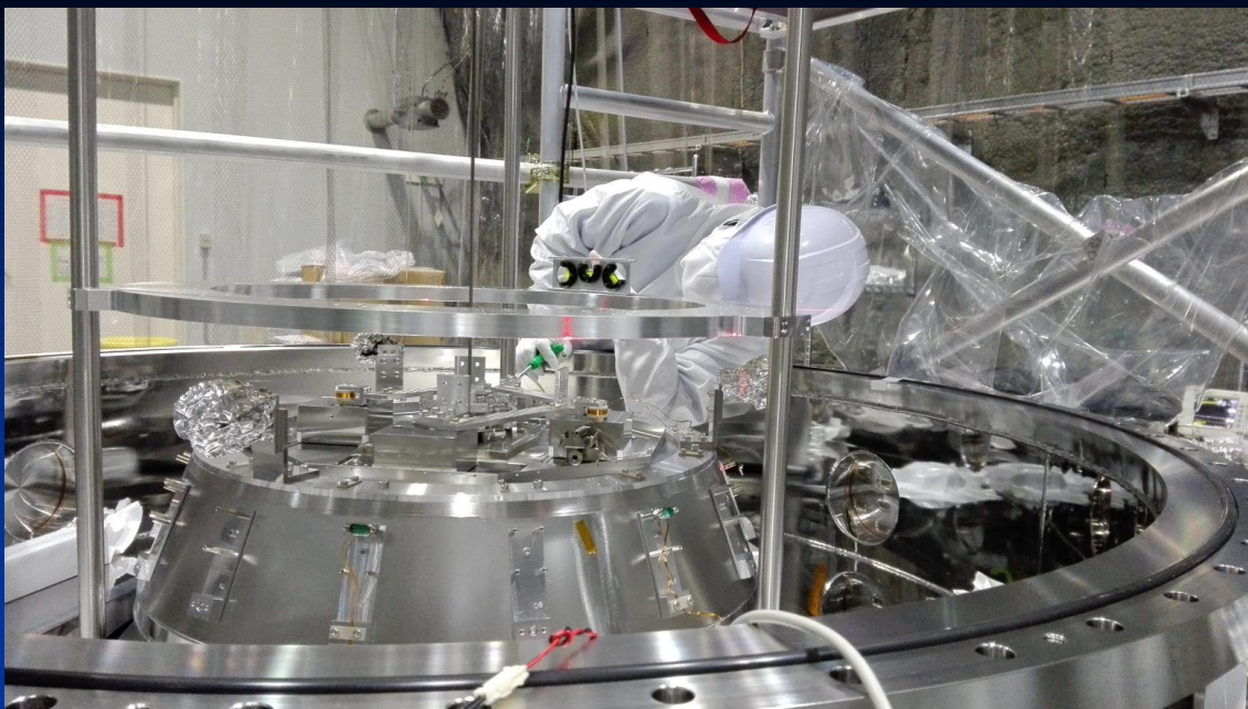
Setting of the bottom filter and the BF damper.
