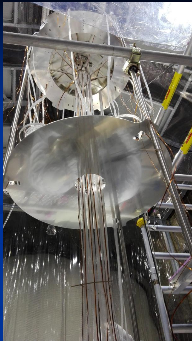
Cabling between the BF and the F3.
