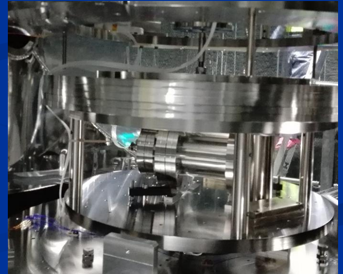
Seismometer on the dummy payload
