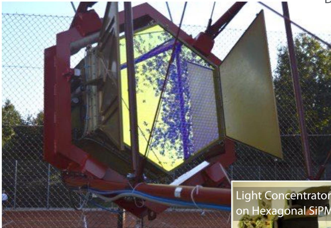
Photon Detection Plane Module
