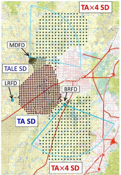
500 SDs, 2.08 km spacing covers ~3x TA SD (about 2100 km<sup>2</sup>) Total about 4x TA SD 3000 km<sup>2</sup> (full operation:2017 Dec -)  $\rightarrow$   $\sim$  12 year TA SD  $\sim$  7 year TA SD from the extension  $\rightarrow$  ~ 19 year TA SD data until 2020 2015 April approved
