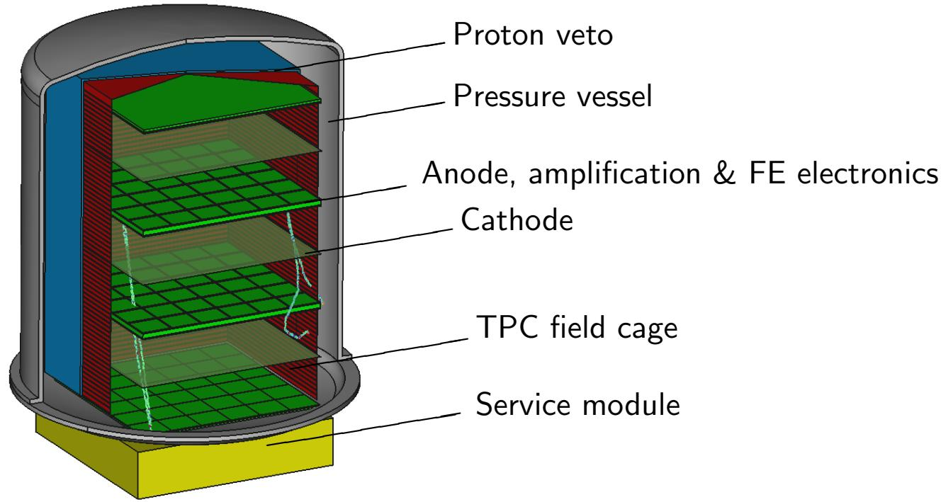
3 layers, each layer of 2 back-to-back modules, each module a  $(2 \text{ m})^2 \times 0.5 \text{ m}$  TPC with an endplate segmented into  $(33 \text{ cm})^2$  micromegas and charge collection blocks. 432 chips,  $(12 \text{ m})^3$ : 100 kg gas at 5 bar.
