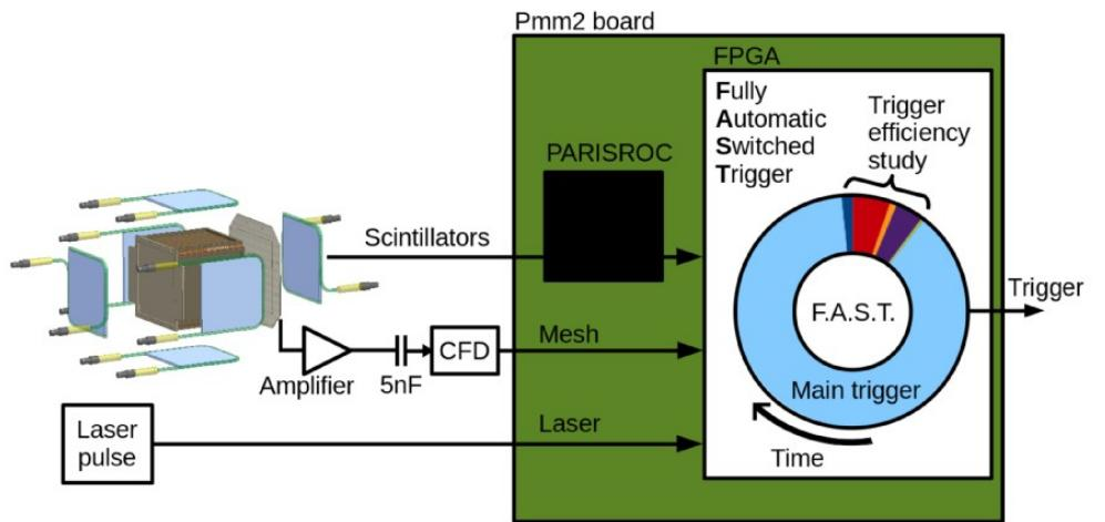
Designed to characterize the performance (signal efficiency, background rejection) of each component of main trigger line
