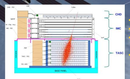
Calorimeter: • Charge Detector • Imaging Calorimeter • Total Absorption Calorimeter • 30 radiation length thickness in total for fully contained events
