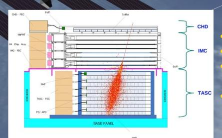
Calorimeter: • Charge Detector • Imaging Calorimeter • Total Absorption Calorimeter • 30 radiation length thickness in total for fully contained events
