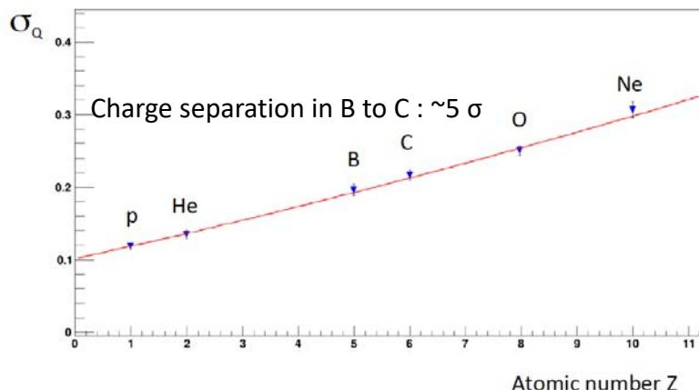
Non-linear response to  $Z^2$  is corrected both in CHD and IMC using a core + halo ionization model (Volz).
