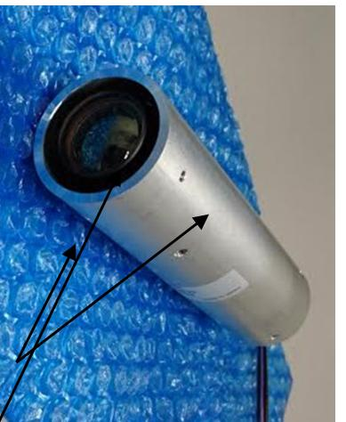
4x  $\Phi 3$  thread (depth 3mm) + Optical grease
