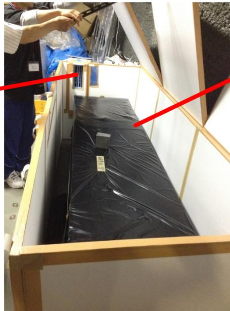
Box made of Lead wall
