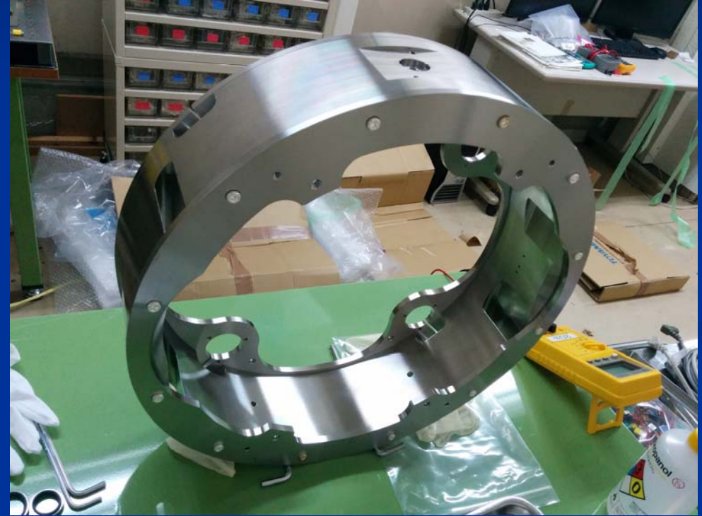
Pre-assembly of the recoil mass (Ti alloy) for BS
