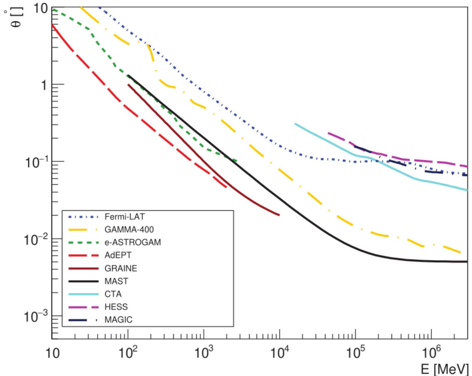
Differential sensitivity for point-like sources: angular resolution is important at low energy! We propose a heavy (~40 t) time projection chamber filled with liquid Argon for Falcon Heavy launcher
