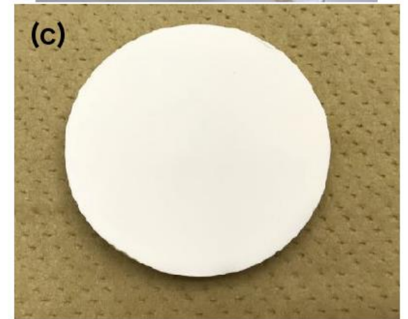
Resin disk 47mm \Phi , 0.5mm T
