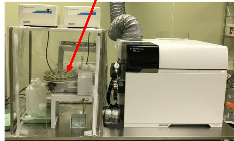
Auto-sampler is covered by clean booth.→Class 100
