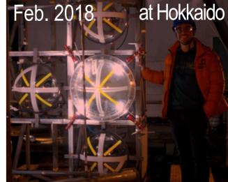
the prototypes passed -9 bar hydrostatic tests
