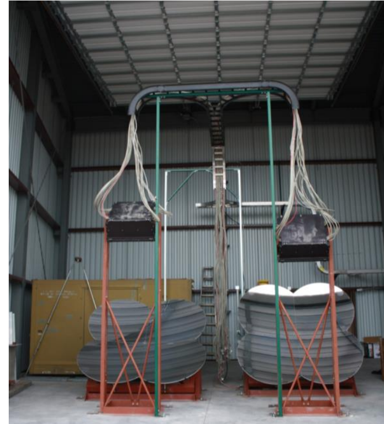
Telescopes for high elevation angle (31-59°)
