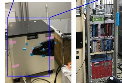
Existing PMT HV and readout electronics
