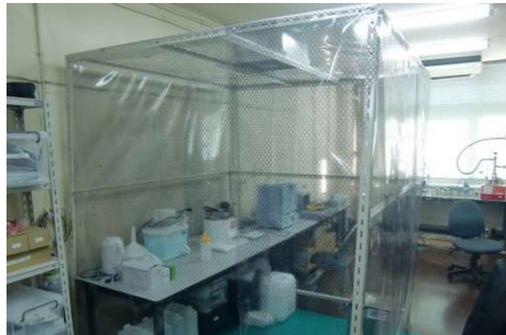
Site for MS development in CST Nihon-U: Clean booth with HEPA filter
