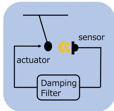
Displacement of the mirror is detected locally by sensors which attached to each stage, and produce a feedback to the mirror actuator with a force proportional to the mirror's velocity.
