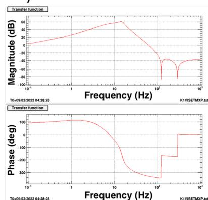
↑ damping filter which we made
